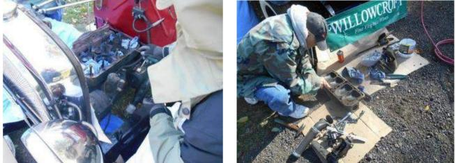
I finish stuffing the holes with rags, while Benny works on the head to scrape off the old gasket.
