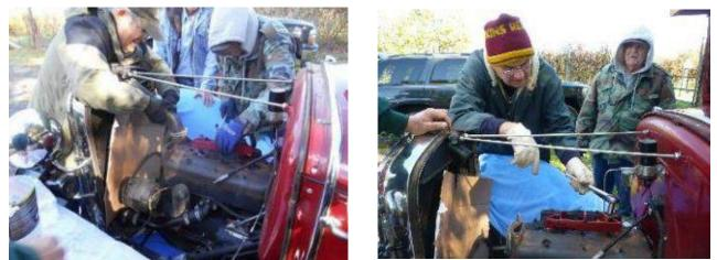
I pull the hose off the goose neck; later, Clem tightens down the nuts on the head puller.
