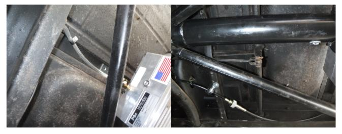
The speedo cable needed a similar approach. The flange on the cross member was very handy to use for the p clamp screw. You can see the plug in the new torque tube for access to the support bearing zerk fitting (one of three new spots to hit with the grease gun.)
