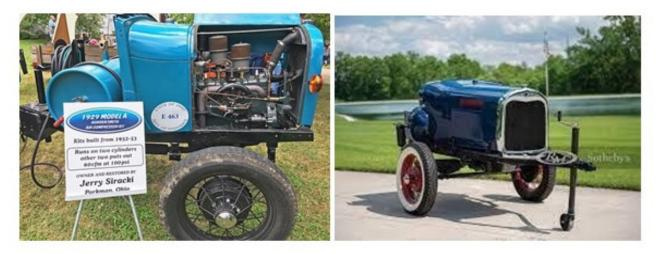
Manufacturer: Engine Horse Power: Max. Air Pressure: Compressor Type: Gordon Smith Company 20 HP. - 90 PSI. - Single Stage - 6 Volt w/positive Ground Fuel Capacity: 11 Gallons Output: 60 CFM. - Air Tank Size: 65 Gals.
