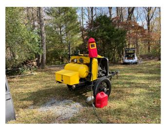
We had a number of problems getting the Smith Compressor to start and, most importantly, stay running at the proper RPM to get the sandblasting gun to operate properly. Luke worked on the distributor while James tackled the carburetor.
