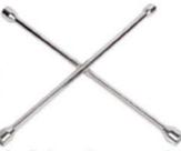
Now slip two of the tire iron arms under the tire, one arm to the left of where the tire touches the ground, and the other arm to the right. Grab one of the tire iron arms that is pointing out toward you, and lift the tire up with one hand while you guide the wheel to hang on a stud or two with the other hand.
