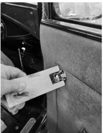
Tool for pushing back the escutcheon so that the pin can be inserted.
