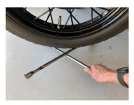
Hold the wheel in against the drum while you lower the lug wrench and use that free hand to start a lug nut on one of the studs. Once you have that lug nut started, you can let go of the wheel and start the rest of them. Use the tire iron to run them all in snug, then lower the jack and tighten them all again.
