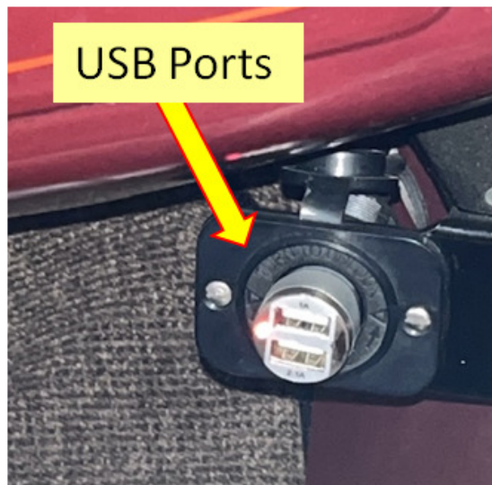
USB ports added to charge cell phones and run a GPS unit
