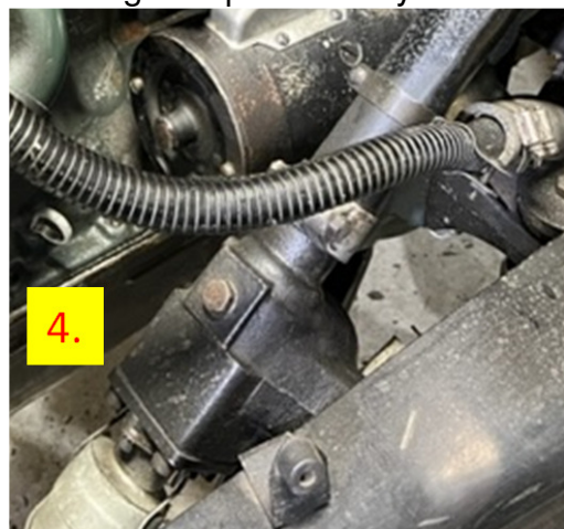
A steering box from a 1987 F-150 steering was installed in place of the Model a version.
