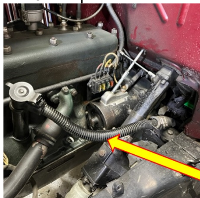
Oil breather tube extends backwards to vent fumes to the rear under the frame
