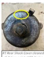
RT Rear Shock Cover cleaned of dirt an paint. HC7 design with AC visible.
