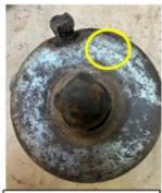
Left Rear Shock Cover cleaned of dirt an paint. HC7 design with CW visible.
