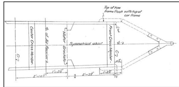
Figure 1. Plan View of Frame with dimensions
