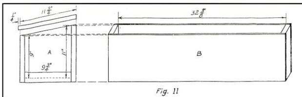
Figure 11. Tool Box & Battery Case
