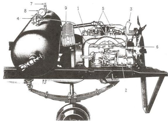
Smith Compressor Components – 1- Special Cylinder Head, 2- Governor, 3- Model B water pump, 4- Pressure Regulator in main tank, 5 – Pressure pistons over reed valves, 6 - Pressure piston on idling device, 7 - Pop-off valve, 8 – Pressure gauge, 9 – intercooler (only on some models)
