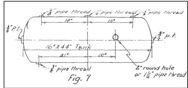
Figure 7. Pressurized Air Tank Dimensions
