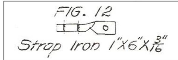
Figure 12. Starter Rod Support
