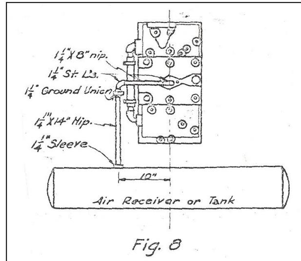
Figure 8. Pressure Tank and Pipe Fittings
