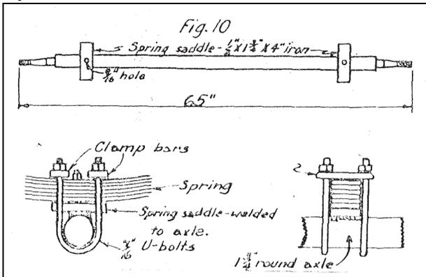
Figure 10. Axle Dimensions and Placement
