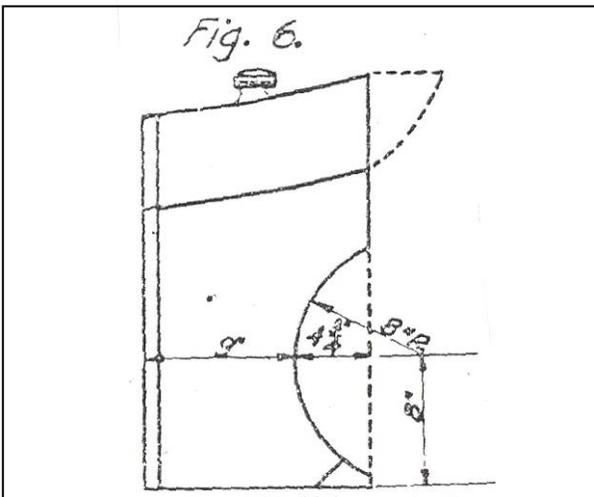
Figure 6. Cowl Tank Cut-out
