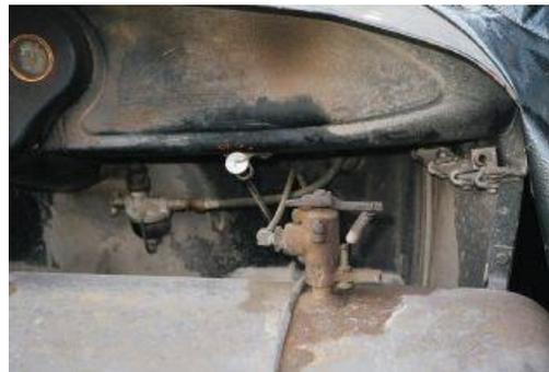
Unloader Pilot Valve on top of tank
