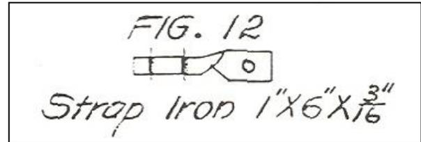
Figure 12. Starter Rod Support
