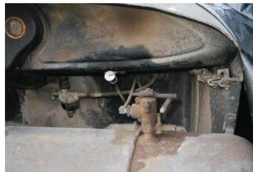
Unloader Pilot Valve on top of tank
