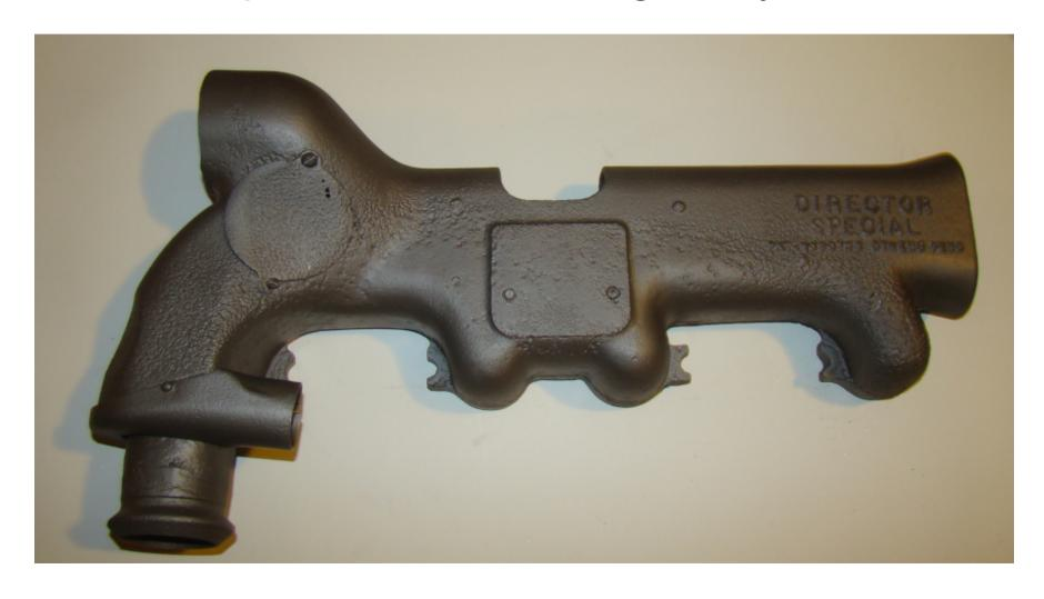
These are somewhat common heaters that were made in both clamp on and special manifold versions. Most of them have the unique feature that the outlet is pointed toward the engine instead of straight back and put an outlet in the center of the firewall. The special manifolds are often confused with Autolite versions since many people don't know the Red Head exists. They are easily spotted though by their angular cover outline as opposed to Autolite's rounded edges.
