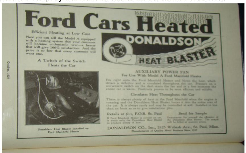
These are probably the most common manifold heaters for Model A. They were made in both clamp on and special manifold styles. Reproduction ones have been made and are not shown here.
