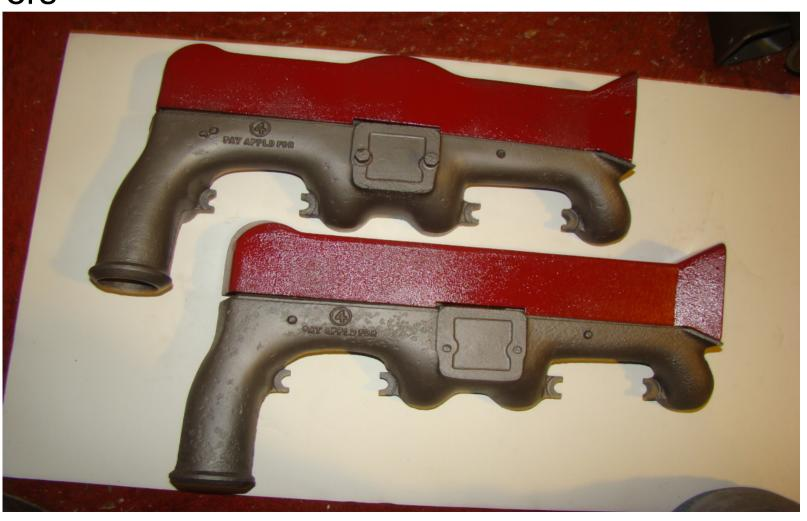
Special manifold style, showing manifold and covers
