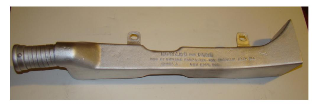
This is a strange unit that is installed between the manifolds and the block and required installing extra long studs to hold it. There are two cast aluminum pieces with a sheet metal cover over both of them. It says "Ford heater model A & B, so this example at least was made after 1931.
