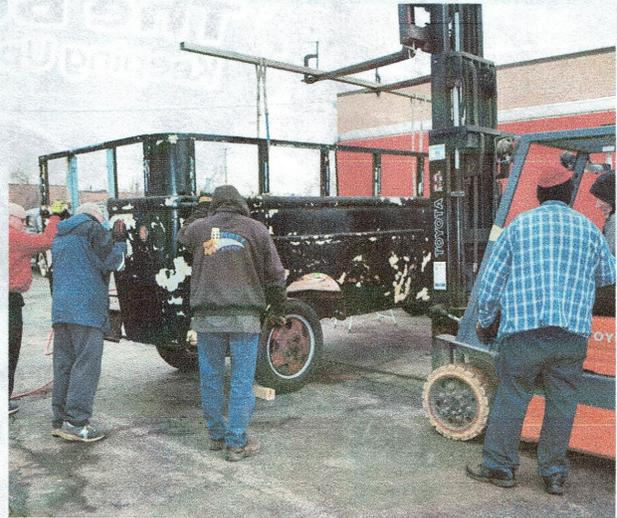
The bus body is now completely apart and is in the process of being stripped sandblasted and moved to a sheet metal shop for the sheet metal repairs to begin. This sheet metal repair is going to cost money as we are going to a restoration shop in Elk Grove Village Illinois. We will do all we can to keep this cost down but this will start to be a large expense for our program.
