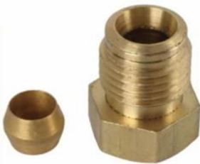
On the bench, before installing anything on the car, slip the tube nut and ferrule on the end of the fuel line like it will be installed on the car. See the photo. Place the ferrule on the tubing with 1/8" of tubing showing on the end. Gently press the nut up against the ferrule and mark that location with a little piece of masking tape.
