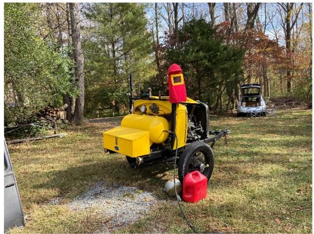
We had a number of problems getting the Smith Compressor to start and, most importantly, stay running at the proper RPM to get the sandblasting gun to operate properly. Luke worked on the distributor while James tackled the carburetor.
