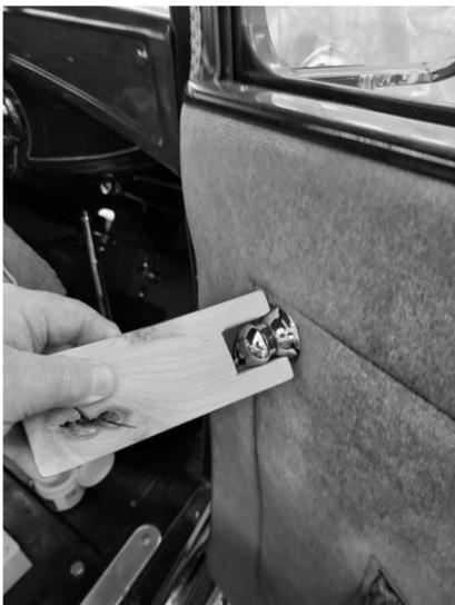
Tool for pushing back the escutcheon so that the pin can be inserted.
