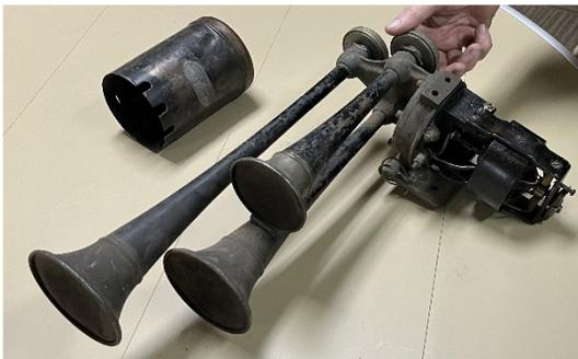
Luke Chapman found a rare functioning Boyce Moto meter that fits onto the steering column of a Model A, it is complete in working order. A non-Model A voltage meter and a Spartan Bugle horn. Luke opened the compressor case of the Horn and explained how it works. He mentioned that he contacted a guy who repairs them and got replacement parts.
