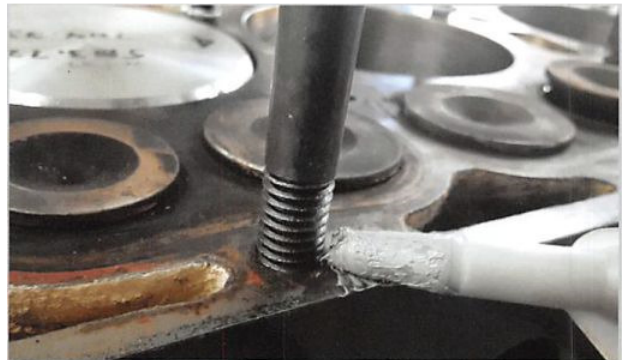
Back stud out 3-4 threads & apply sealer sparingly to exposed threads.
