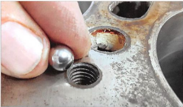
Drop one ball into the head stud hole. This is to prevent the stud from bottoming out on the end of the threads.
